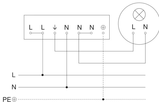
Connection using two-circuit switch for manual and automatic operation
