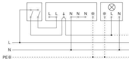
Connection via a two-way switch for manual override and automatic operation
